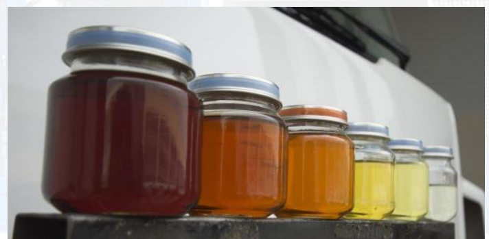
Transformer oil in various stages of the oil regeneration process
